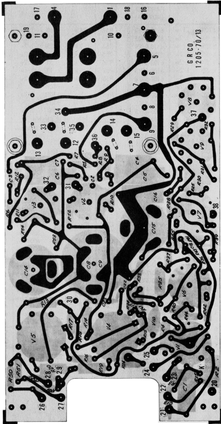
Figure 6. Etched Board Layout Diagram.
