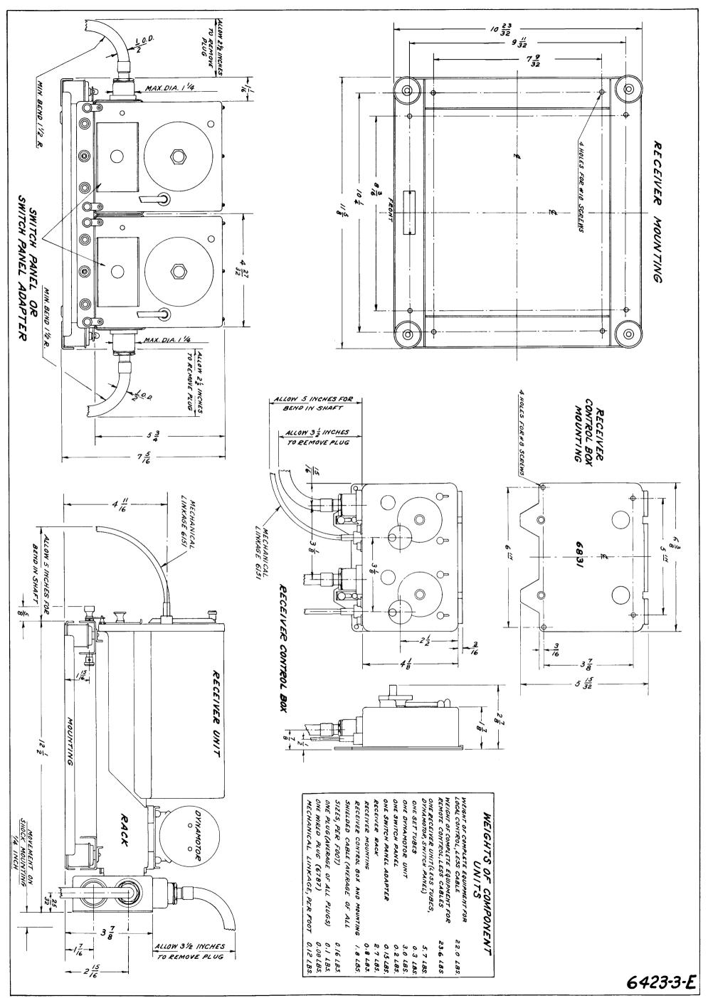
Fig. 13—Installation Dimensions and Weights, Units of Model RAT and Model RAT-1 Equipment
