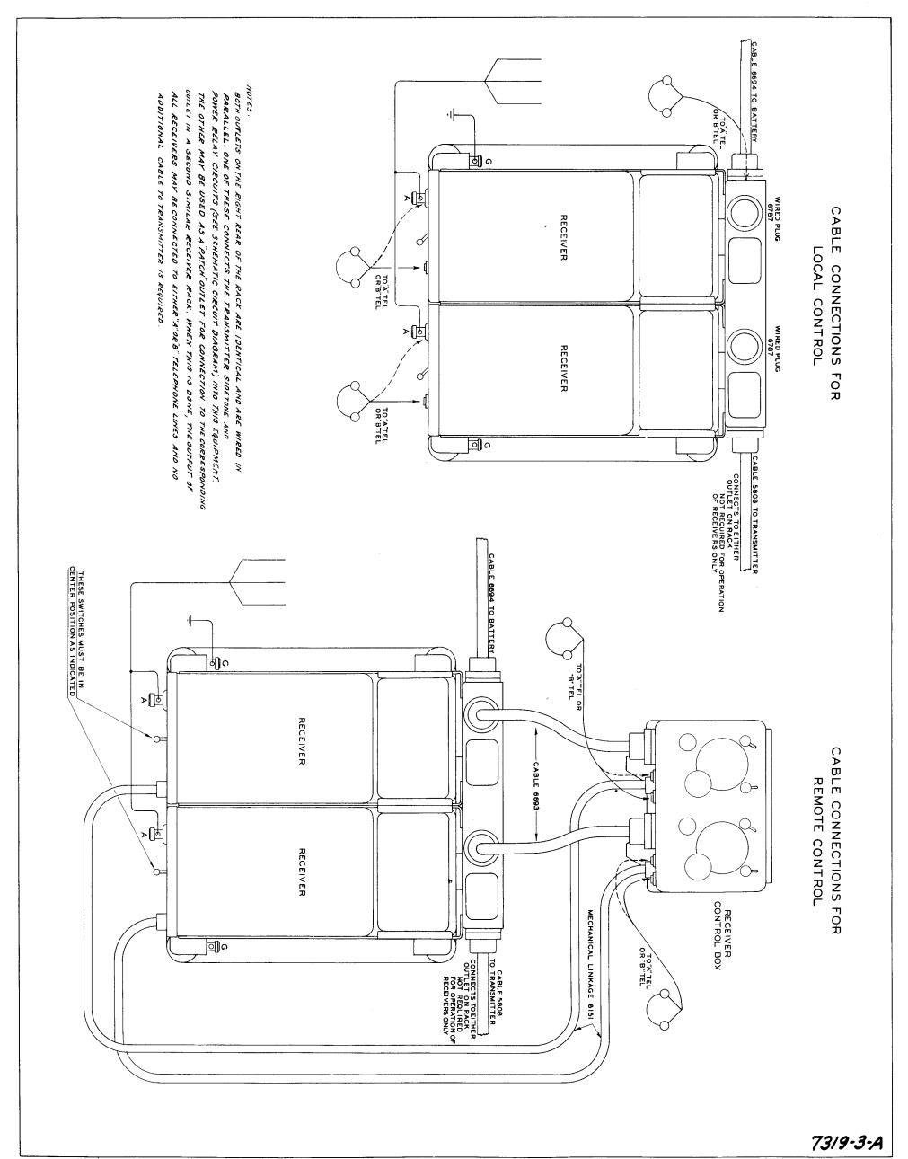
Fig. 12—Cabling Diagram, Model RAT and Model RAT-1 Equipment
