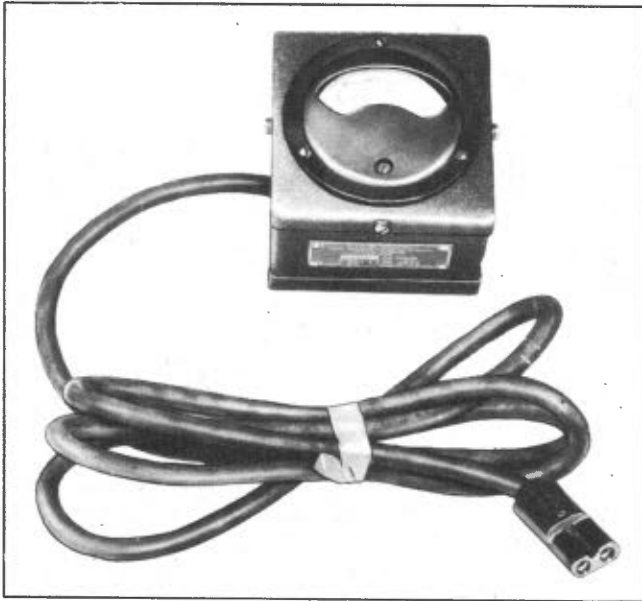
Figure 2-6. Test Set I-139-A—External View
